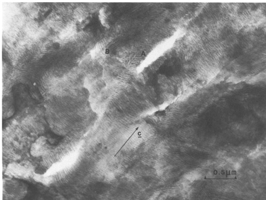
Figure 1 Lamellar texture in a stained microtome section of single-crystal texture polyethylene. In this and all subsequent figures the plane of the electron microscope specimen is parallel to the plane of the compressed sheet, i.e. the preferred (1 0 0) plane orientation.
